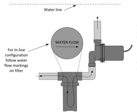
In this configuration it is critical that the filter canister is oriented in an allowable orientation (see above). The filter must be able to self purge air pockets else there may result an air lock in the pump. When mounting in a pond a pre-strainer sponge is also be connected to the filter inlet as a secondary filter. If required.
