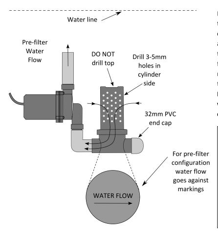
Before mounting the pre-filter you need to drill 3-5mm holes in the side of the cylinder (DO NOT drill top). The size of and number of these holes will depend on the application. The internal mesh will form a secondary filter. You may also require a pond sponge wrapped around the cylinder depending on the application. **Note water flow goes against the actual water flow markings on the filter for this configuration.**
