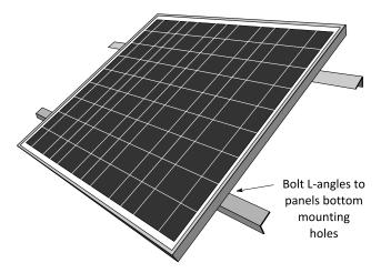
1) If mounting on a roof we recommend a 20-30mm air gap be used between the solar panel and roof structure. Aluminium angles (20-30mm) should be attached to the back of the solar panel for mounting purposes using the back mounting holes. **Important: Wind loading should be considered.**
